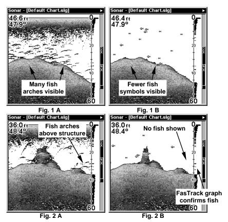
Figures 1A and 2A (left) show Sonar Page in normal chart mode. Figures 1B and 2B (right) show the same underwater scene with Fish I.D. turned on. Note how arches are replaced with symbols.
